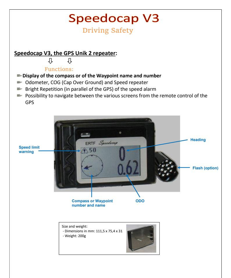
*More functions:* The V3 *Eue* version of Speedocap V3, equipped with a GPS module, works off-line (when you are not connected to GPS Unik 2).
